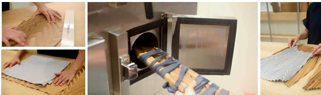
Left to Right: Processes of UNWAKE by GINLEE Studio that includes pleating and steaming of the pleated product. Images by GINLEE Studio.
